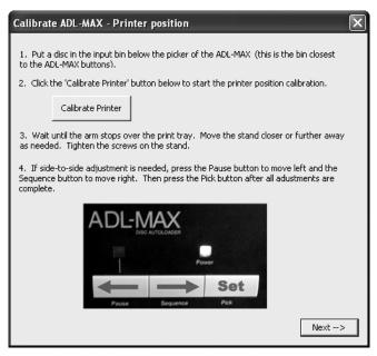
You can recalibrate at any time by opening Primo DVD -Click the robotics menu - select options - Click the Calibrate ADL-MAX button. If you are using RoboPrint, click Robot Options - Calibrate ADL-MAX.
